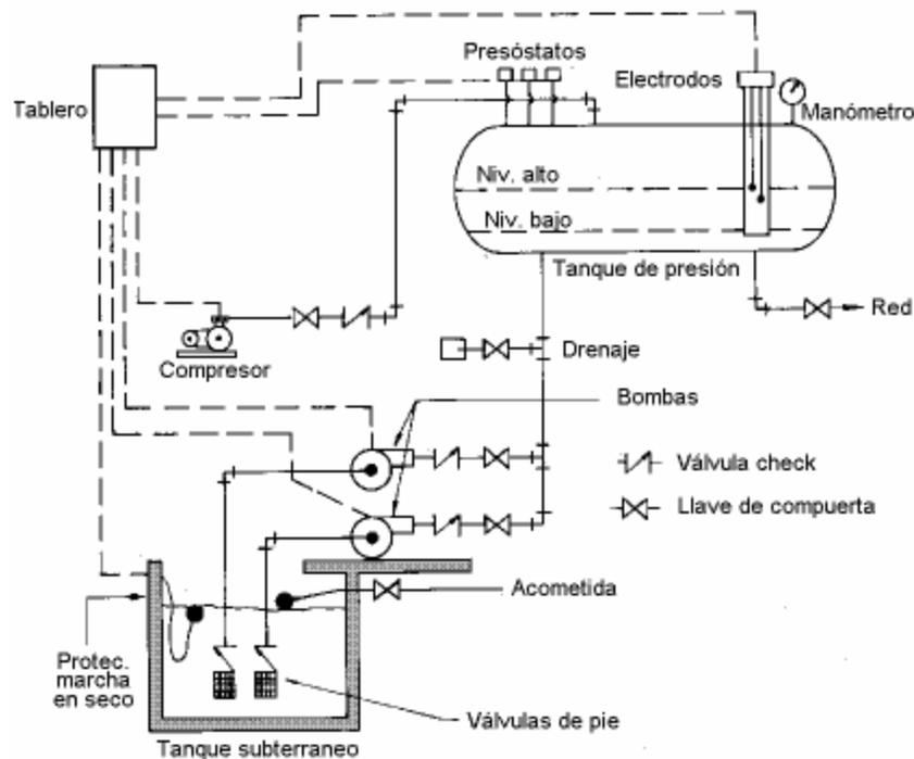
Figure 1: Diagram of a hydropneumatic system.
